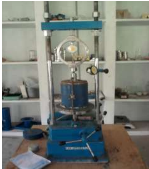
Figure: 3 California Bearing Ratio Test Apparatus
